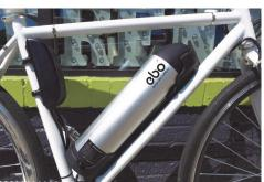
the screws to fix the battery holder to the frame. Put the battery into the case, turn off battery and lock the battery.
