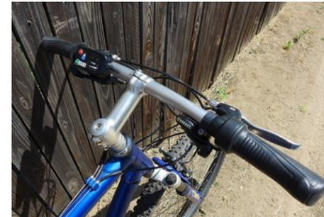
handlebar grips (use Isopropyl Alcohol).
