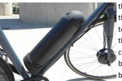
the screws to fix the battery holder to the frame. Put the battery into the case, turn off battery and lock the battery.
